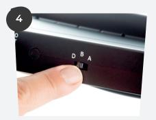
**Step four** Select a channel to the transmitter.
