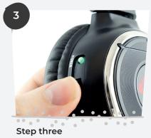
Tapping the power button to change channel. The LED light will change according to the channel.
